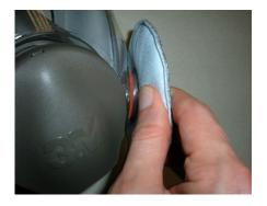
Filter Installation – What NOT to do Hold aggressively, or on seam
